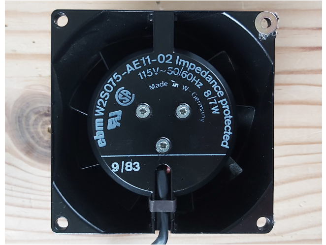
Figure 1.1: Adjust the blade assembly screws.
